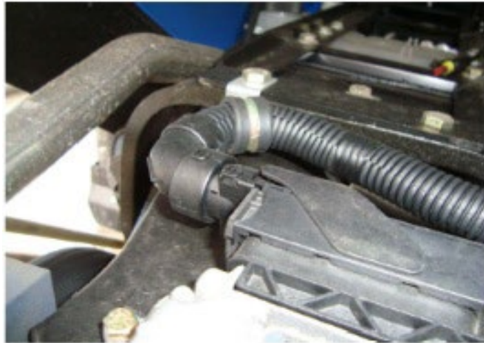
Figure 3: Example of wiring harness layer (distance \leq 150 mm, same vibration level)
