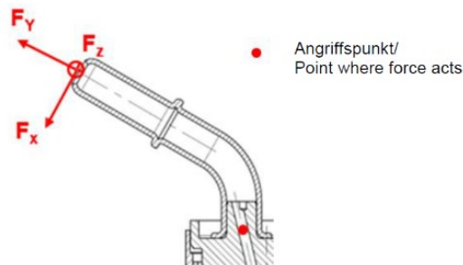
Figure 7-24 Force at DEF- hydraulic connector
